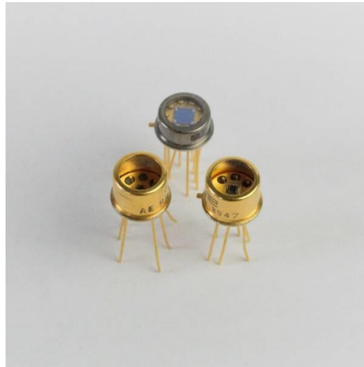
Silicon photodiodes in TO-housing
